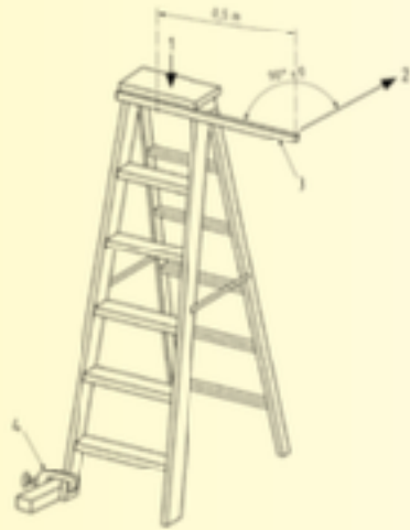
a) Torsion test for standing step ladders
