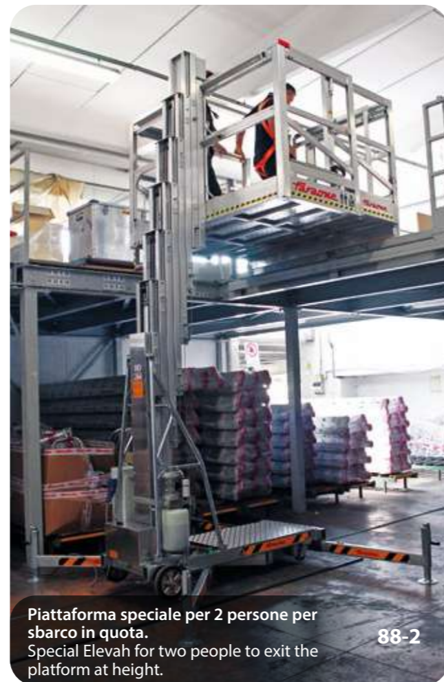
Elevah speciale per sbarco in quota. Special Elevah designed to exit the platform at height.
